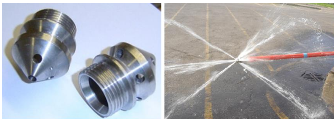
Victor 喷枪，来源“Cheshire”事故调查报告 (Isle of Man Ship Registry)
