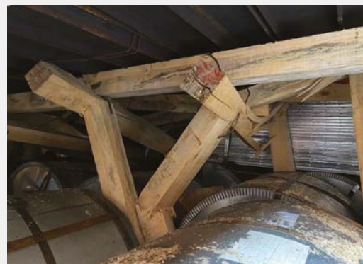
Inappropriate or Insufficient Dunnage Between the Cargoes
