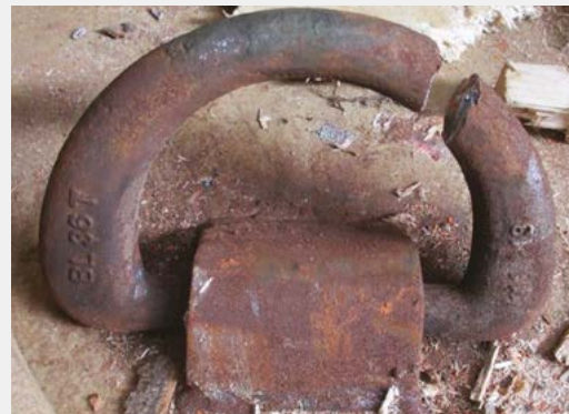
Multiple Lashings Attached to a Single Securing Point, Exceeding the SWL
