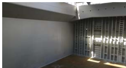
Up: Single Hull Plate More Vulnerable to Sweat Bottom: Double Hull Plate Less vulnerable to sweat
