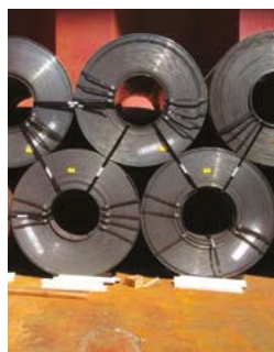
Dunnage Too Short
