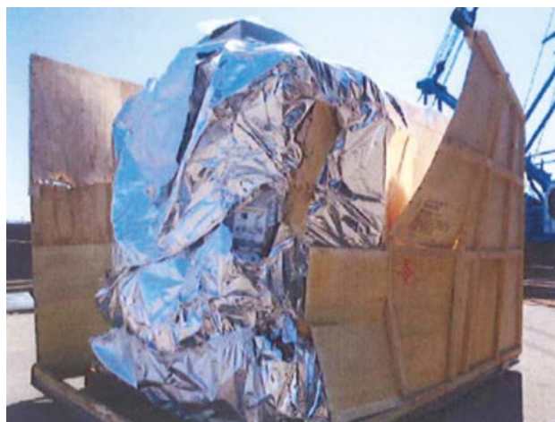
Damage Due to Improper Packing
