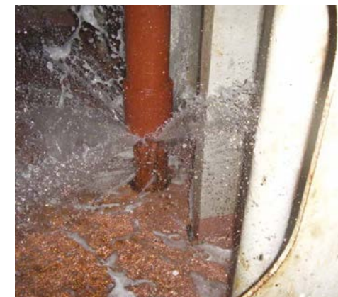
Right Picture (from top to bottom) Leaking Manhole Cover Leaking Tanktop Bunker Leaked into Cargo Hold Through Damaged Sounding Pipe Sounding Pipe Leakage
