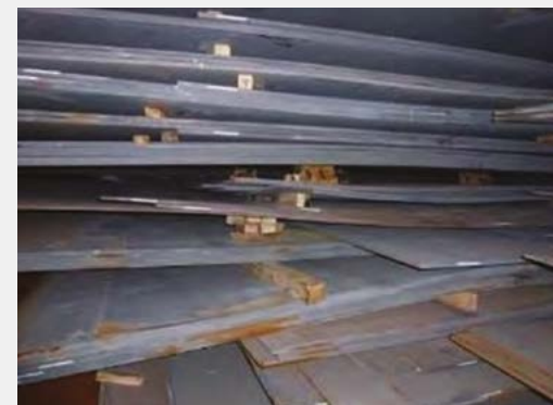
Dunnage for Steel Plates not Vertically Aligned
