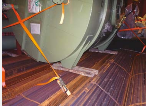
Insufficient Lashing, Inappropriate Size of Lashing Materials, and Incorrect Lashing Angles
