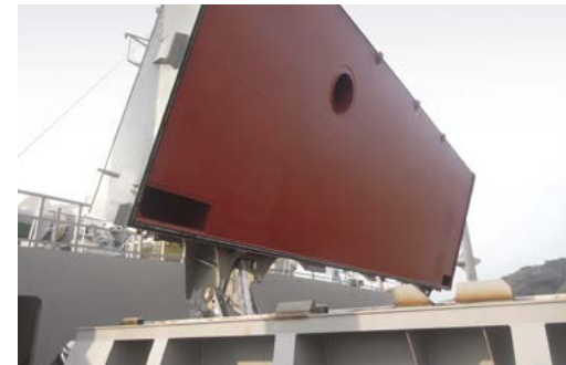
Double Skin Hatch Cover Less Vulnerable to Sweat
