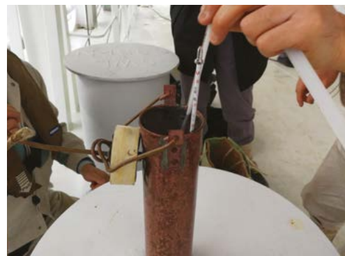
Testing the Seawater Density
