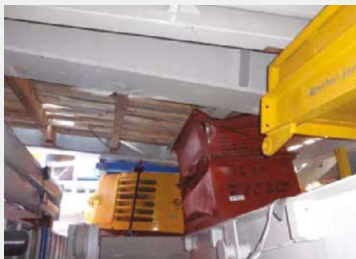
Heavy Cargo Stowed on Top of Light or Fragile Cargo (Source: The America Club)
