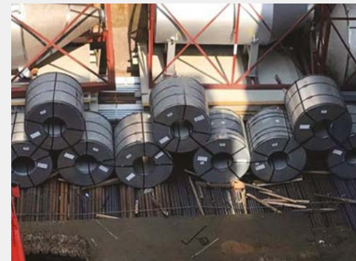
Coiled Sheet Steel Stowed on Top of Other Cargoes
