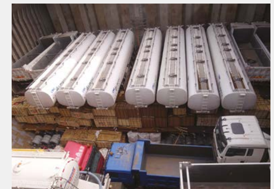
Wheel-Based Cargoes or Heavy Cargo Items Stowed on Top of Bagged Cargoes or Cargoes Without a Solid Base
