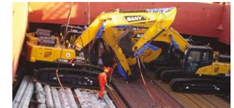
Loaded on Top of Other Cargoes Without Dunnage
