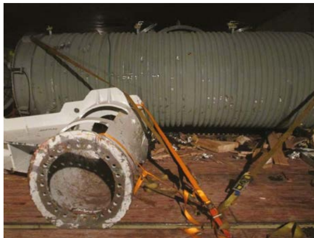
Damage Due to Improper Stowage and Lashing
