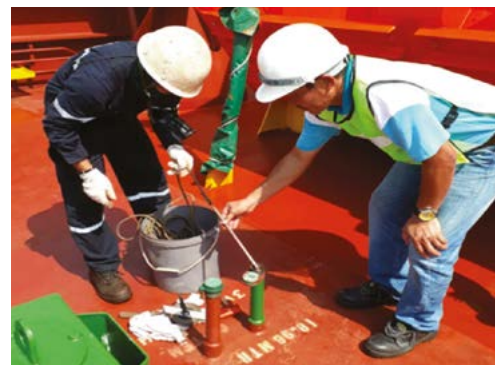
Sounding the Tank
