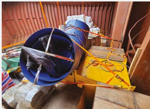
Securing Points on the Ship and/or on the Cargo are not of Adequate Strength
