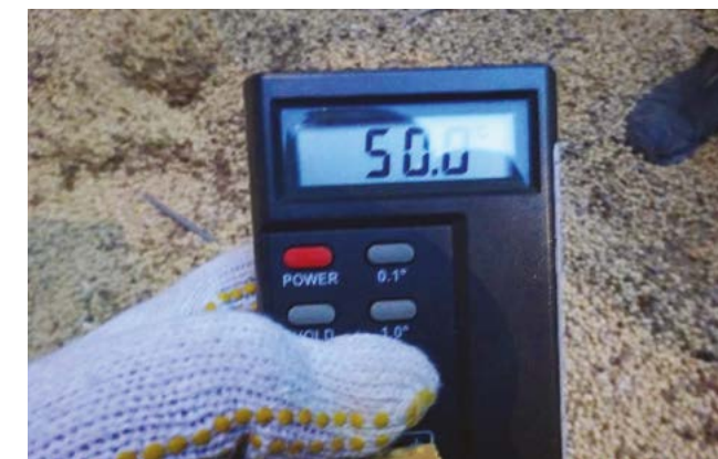
The Temperature of Cargoes Close to Fuel Tank
