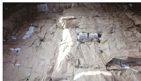
Kraft Paper Covered on Bagged Cargoes
