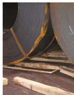
Dunnage Too Soft and Crushed (Source: The America Club)
