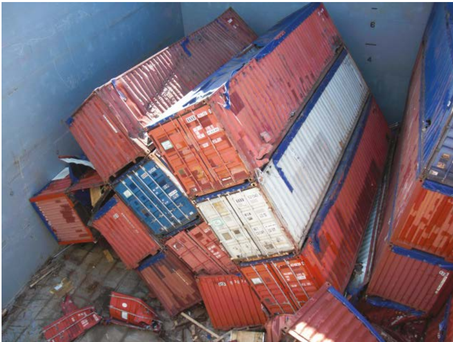
Container Stacks Collapsed in Cargo Hold
